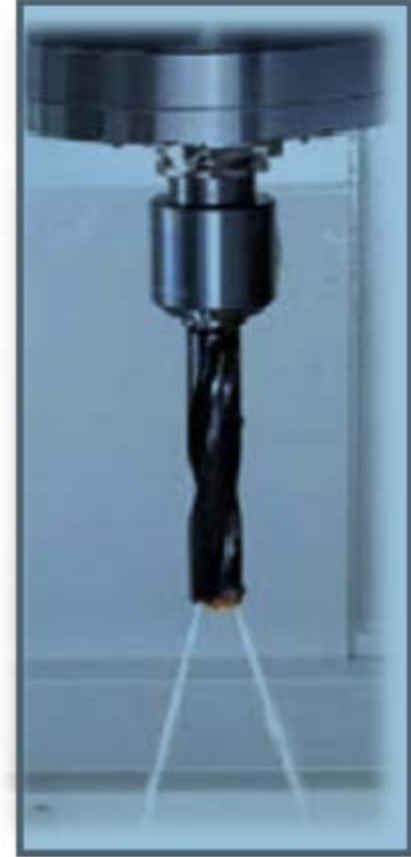
Tool center water outlet
