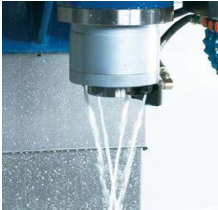
Spindle annular spray cooling
