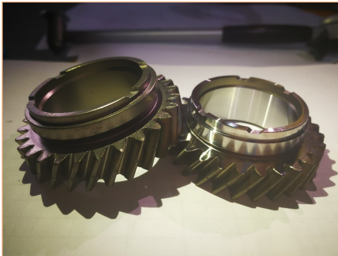
Hard turning after gear heating
